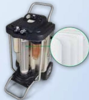
The **UNGER RO** utilizes 3 stage water purification system. First, the combi-pre-filter captures chlorine and sediments from the incoming water, then the water is directed towards 2 RO membranes which remove up to 98 % of dissolved minerals and contaminants.
