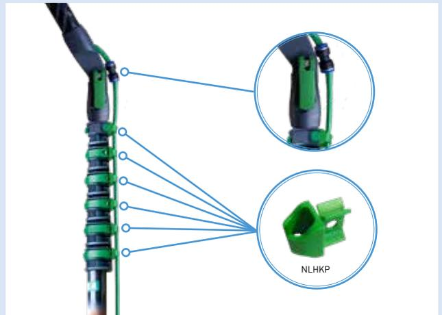
Fit hose clips NLHKP into the clips of the nLITE telescopic pole. Guide the hose through the clips on the outside of the pole and connect it to the angle adapter using the quick connector on the angle adapter.
