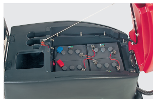
Machine open showing the batteries
