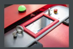
7-inch touchscreen (HMI) Easily control your robot using the large and user-friendly touchscreen (HMI).
