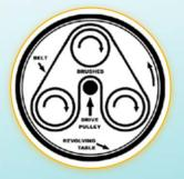
The triple-brush cleaning mechanism incorporates a contra-rotating planetary drive disc
