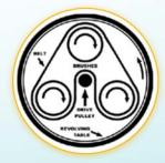
The triple-brush cleaning mechanism incorporates a contra-rotating planetary drive disc
