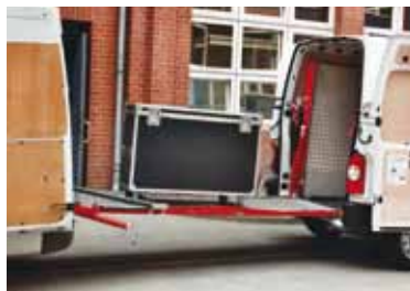
RAMP FOR DOCK LOADING 450 Kg
