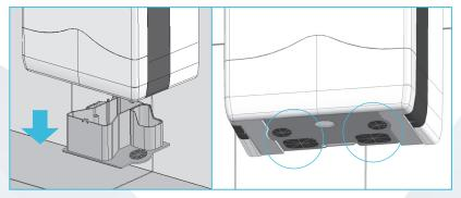
The basic maintenance consists in emptying the water tank and cleaning the air filters following the instructions of the user's manual.
