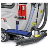
KIT FOR CLEANING ACCESSORIES For bringing additional cleaning tools with you, which are useful for completing the operations (upon request)
