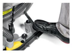
The brush head is lowered/lifted through a comfortable pedal (Version without PM-Pressure Monitoring)
