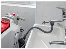
The hose for filling the solution tank can be connected directly to any water tap, thus allowing the machine to be quickly refilled at any location
