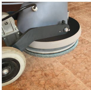
Example of usage on marble surfaces, from roughing with diamond-coated metal grinding disc to high gloss polishing with TMB SHINEPAD disc
