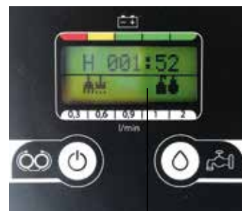
Residual runtime and hour counter
