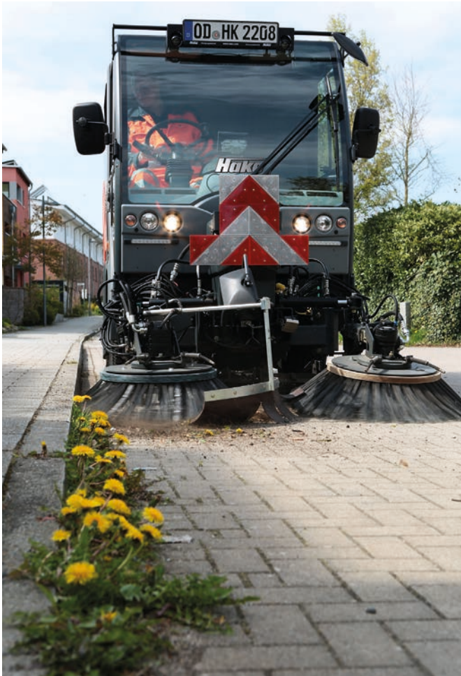
For the powerful mechanical removal of weeds, light weed brushes are used, which can be fitted quickly and easily. (Photo: Hako)
