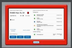
7-inch touch screen (HMI) The user-friendly and purpose-designed control unit directly built into the robot.
